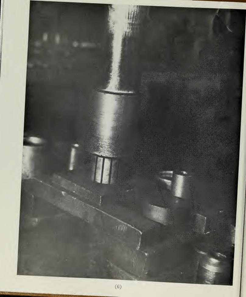
Any errors in the mounting of the core or commutator on the shaft are corrected by means of adjusting their respective placements by means of an arbor press. The laminations of almost every core are pressured together on this same press before any further steps are taken. This latter operation (illustrated above) is done to realign any laminations which may have become somewhat separated.
